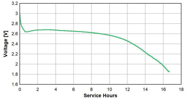
Pulse Discharge 10mA 5s/m, 24hd until 1.8V
